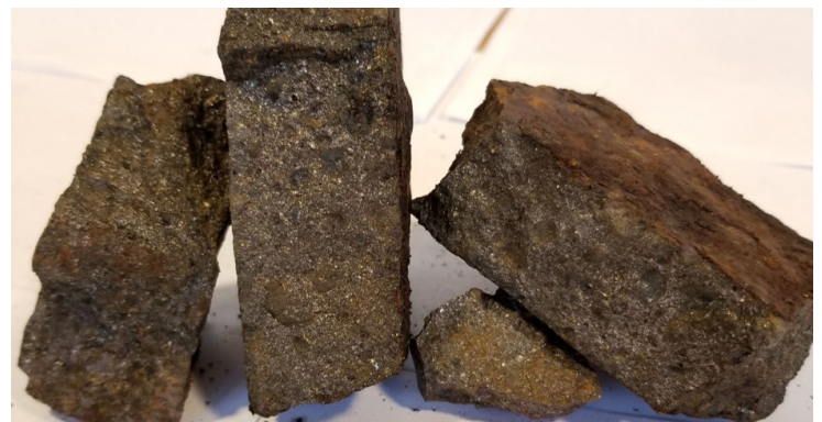
Semi-massive to net-textured pyrrhotite with trace chalcopyrite in gabbro/gabbro-norite (cliff gossan zone)
